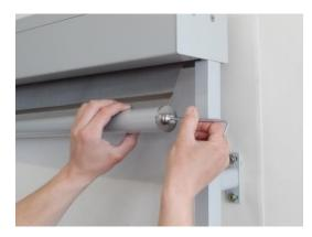
2. Connect the drive to power supply and unroll the fabric, then unscrew the bolts in the bottom bar that are used to assemble the movable part of the arm.
